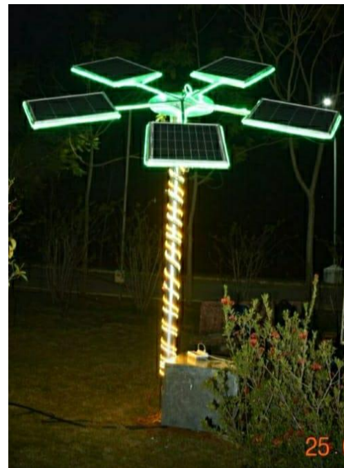
Fig.3. developed solar tree for EV charging
